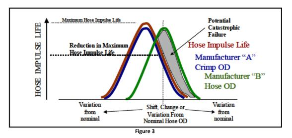
You can see from Figure 3 that even in the best-case scenario, you have significantly reduced impulse performance as compared to a Gates hose assembly that is designed as a system and validated through a rigorous test regiment. As Figure 4 shows, things get even worse when you take a look at all the variables.
