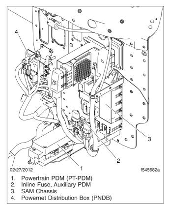
Fig. 3.3, Engine Compartment Power Distribution Components
