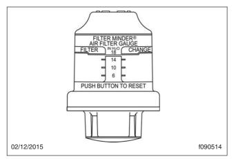
Fig. 4.6, Air Intake Restriction Indicator
