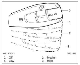
Fig. 13.7, Engine Brake Positions, Detroit Multifunction Control
