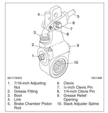
Fig. 21.1, Gunite Automatic Slack Adjuster
