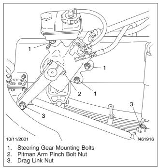
Fig. 21.18, Integral Steering Gear Fasteners
