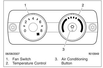
Fig. 5.38, Sleeper Climate Control Panel
