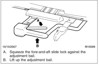
Fig. 7.6, Fore/Aft Slide Adjustment, Sears Atlas Seat
