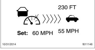
Fig. 6.23, ACC Lead Vehicle Detected (green)
