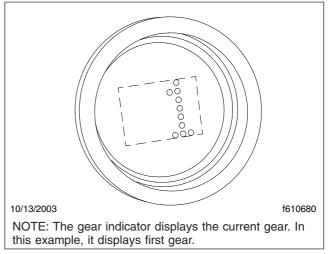
Fig. 15.10, Current Gear Display
