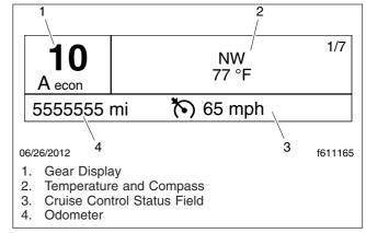
Fig. 4.23, Driver Message Center with Gear Display, ICU4Me
