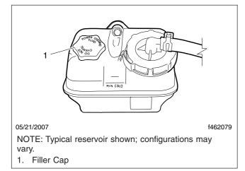
Fig. 21.5, Power Steering Fluid Reservoir
