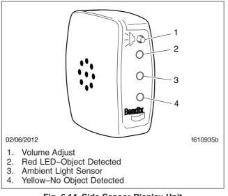
Fig. 6.14, Side Sensor Display Unit
