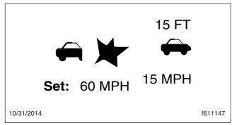
Fig. 6.24, ACC Collision Warning (red)
