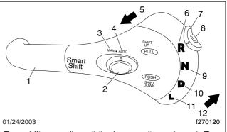
To upshift manually, pull the lever up (towards you). To downshift manually, push the lever down (away from you).
