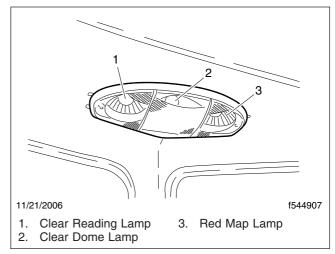
Fig. 5.9, Overhead Console Lights
