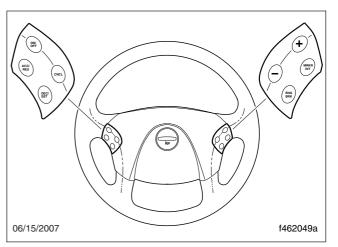
Fig. 13.5, Steering Wheel Switches
