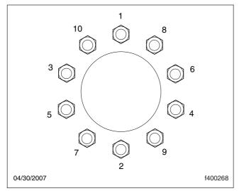
Fig. 21.4, Tightening Pattern, 10-Hole Wheels
