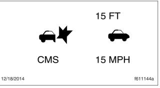
Fig. 6.21, CMS Collision Warning (red)
