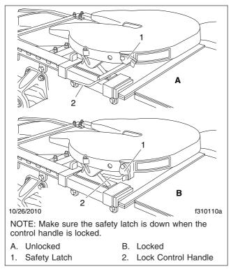
Fig. 18.2, Fontaine Locking Mechanism
