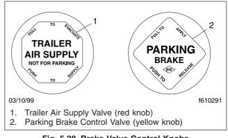
Fig. 5.28, Brake Valve Control Knobs
