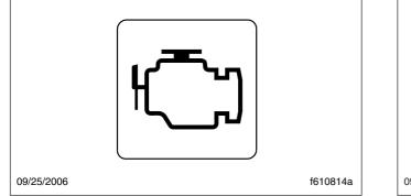
Fig. 12.4, Malfunction Indicator Lamp (MIL)
