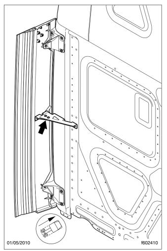
Fig. 24.7, Side Extender Middle Bracket
