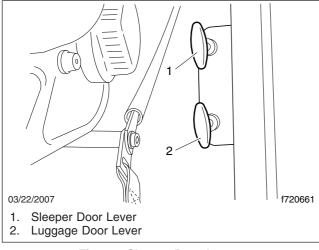
Fig. 2.6, Sleeper Door Levers
