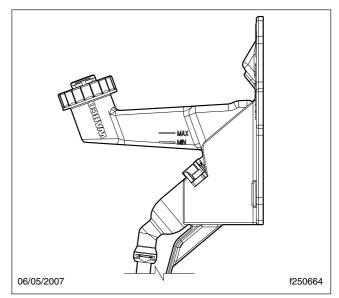
Fig. 14.4, Clutch Fluid Reservoir
