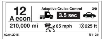
Fig. 6.29, Adaptive Cruise Control Screen
