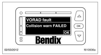
Fig. 6.15, VORAD Fault Display
