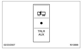
Fig. 5.35, Trailer Auxiliary Switch
