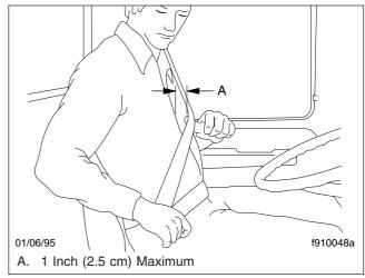
Fig. 7.11, Adjusting Shoulder Harness Clearance, Komfort Latch
