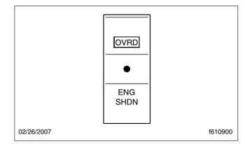
Fig. 11.2, Shutdown Override Switch
