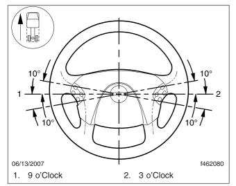
Fig. 17.1, Proper Steering Wheel Position (with tires pointed straight ahead)
