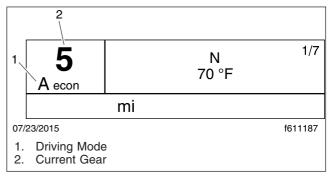
Fig. 15.2, Gear Display Window
