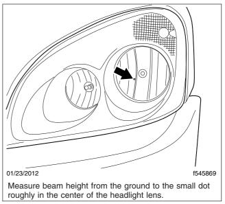
Fig. 23.1, Headlight Beam Height Adjusting Dot
