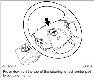
Fig. 5.13, Steering Wheel With Airbag
