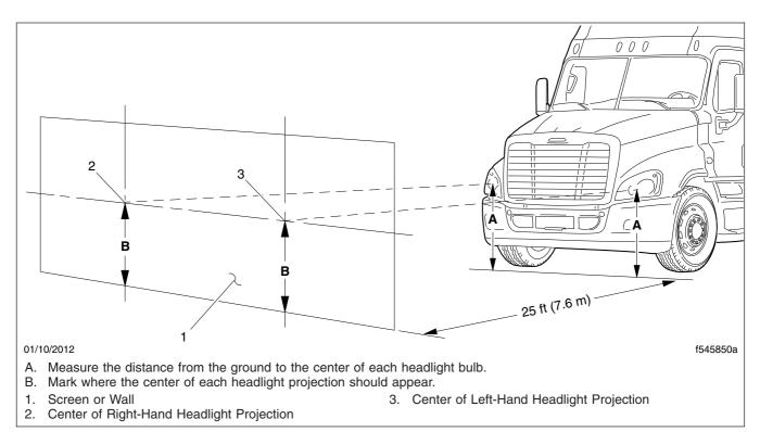
Fig. 23.2, Headlight Aiming Screen/Wall
