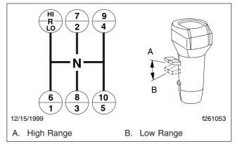
Fig. 14.3, Eaton Fuller 10-Speed Transmission Shift Patterns
