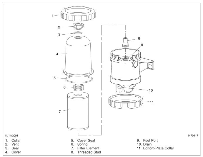
Fig. 24.3, Davco Model 382 Fuel/Water Separator
