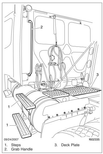
Fig. 2.7, Back-of-Cab Access
