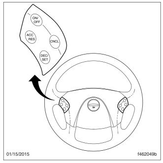
Fig. 6.28, Steering Wheel Cruise Control Switches
