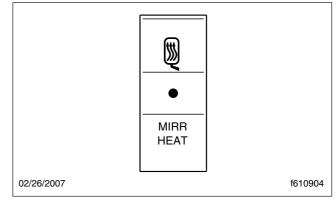
Fig. 9.2, Mirror Heat Switch
