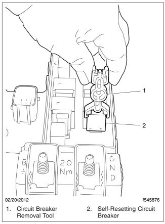
Fig. 3.5, Self-Resetting Circuit Breaker Removal
