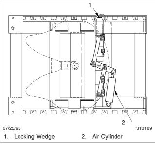
Fig. 18.15, Air-Operated Sliding Fifth Wheel (Fontaine shown)
