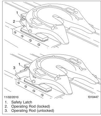
Fig. 18.3, Holland Simplex SE Locking Mechanism
