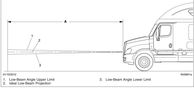
Fig. 23.3, Vertical Low-Beam Headlight Variation Limits
