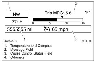
Fig. 4.22, Driver Message Center Without Gear Display, ICU4Me
