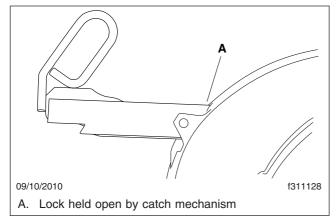
Fig. 18.7, Jost Release Handle Unlocked
