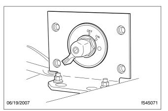
Fig. 3.6, Cab Load Disconnect Switch, EPA07
