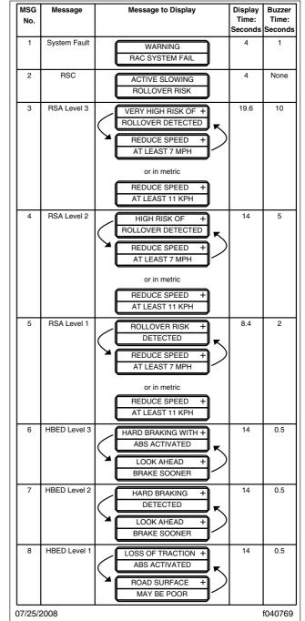
Fig. 6.37, Roll Stability and Hard-Braking Warnings
