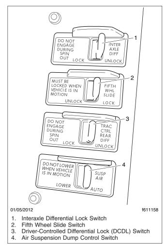
Fig. 5.15, Axle and Suspension Switches
