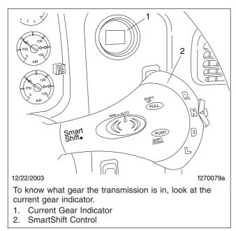
Fig. 15.7, Shift Controls and Indicators, UltraShift Transmissions
