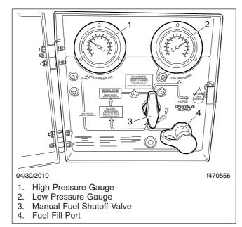
Fig. 21.10, CNG Fuel Panel
