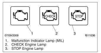
Fig. 11.1, Engine Warning Lamps
