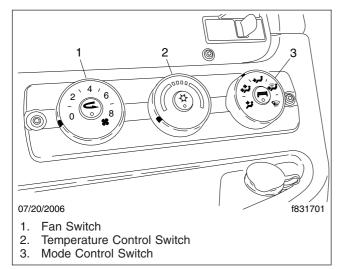
Fig. 8.1, Cab Climate Control Panel
