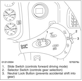
Fig. 15.9, Switches, UltraShift Transmissions
