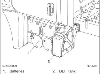
Fig. 12.7, DEF Tank Located Behind the Battery Box
