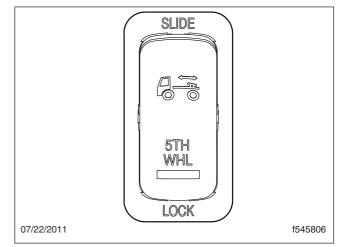
Fig. 5.34, Fifth Wheel Slide Control Switch
