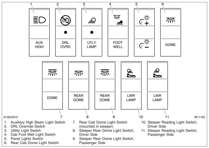
Fig. 5.4, Dash-Mounted and Sleeper-Control Light Switches
