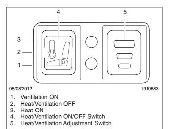
Fig. 7.3, Cascadia 2.0 Hi-Back Seat Heat/Ventilation Controls
