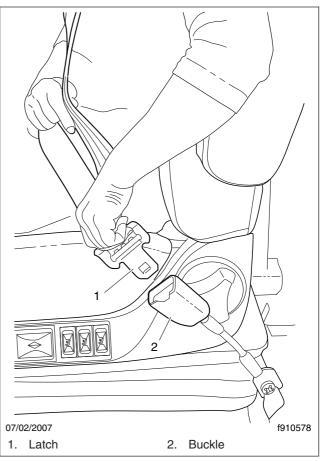
Fig. 7.9, Three-Point Seat Belt Operation
