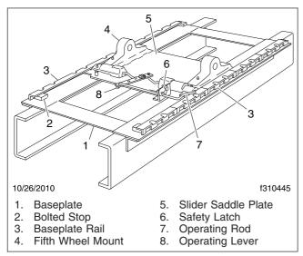
Fig. 18.13, Sliding Fifth Wheel Manual Release, (Holland Simplex)
