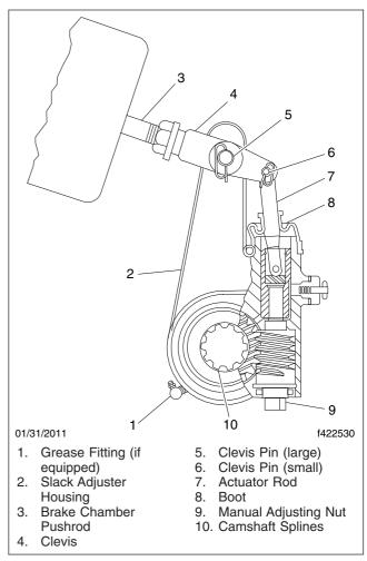
Fig. 21.3, Meritor Automatic Slack Adjuster
