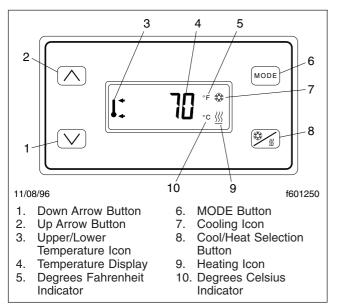
Fig. 11.4, Optimized Idle Thermostat
