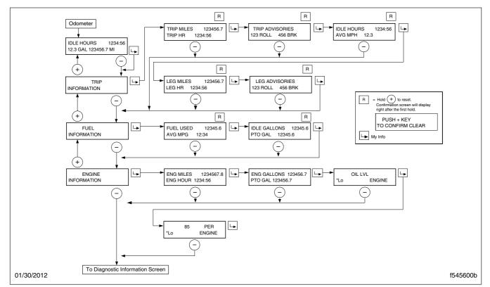
Fig. 4.17, ICU4M Idle Hours, Trip Information, Fuel Information, and Engine Information Screens
