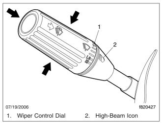
Fig. 5.8, Multifunction Turn Signal Lever
