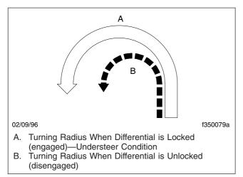
Fig. 16.1, Turning Radius
