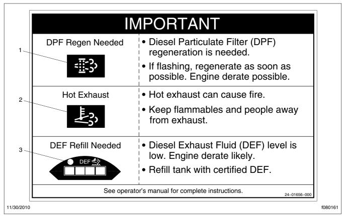
Fig. 12.2, Warning Lamp Decal, Sun Visor
