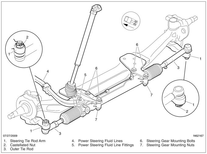
Fig. 21.17, Rack and Pinion Steering Gear Assembly
