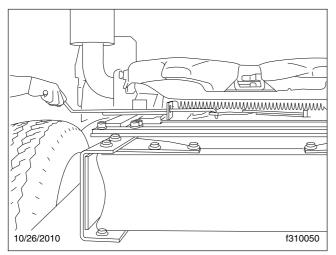
Fig. 18.12, Releasing the Sliding Fifth Wheel, (Fontaine)
