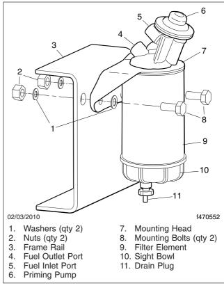
Fig. 21.15, Alliance Fuel/Water Separator Assembly and Installation
