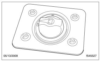
Fig. 3.7, Cab Load Disconnect Switch, EPA10 and Newer
