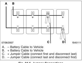
Fig. 24.5, Jumper Connections
