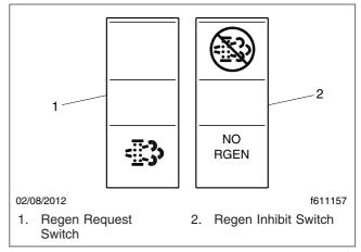
Fig. 5.14, Regen Request and Inhibit Switches
