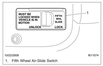
Fig. 18.14, Air-Slide Switch
