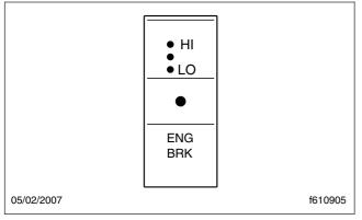
Fig. 5.16, Engine Brake Switch
