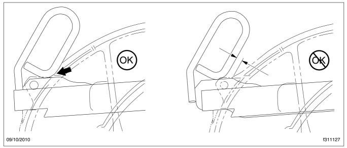
Fig. 18.8, Jost Release Handle Locked
