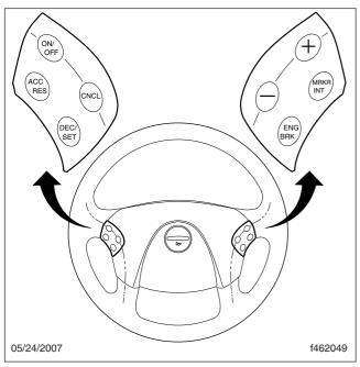
Fig. 5.7, Steering Wheel-Mounted Controls
