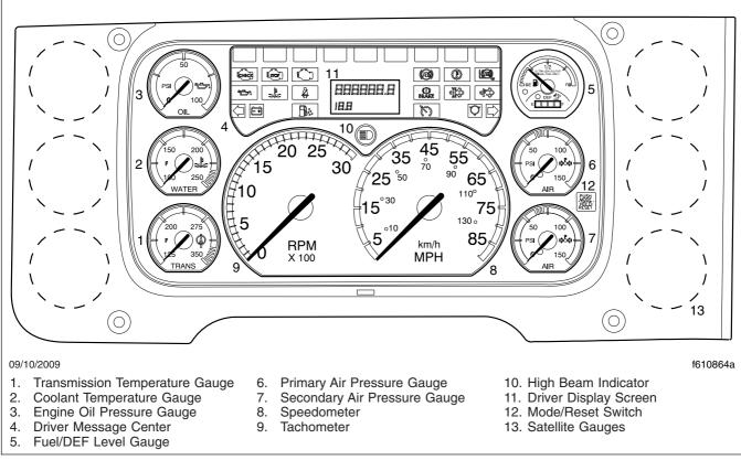
Fig. 4.1, ICU3 Instrument Cluster (EPA10 shown)
