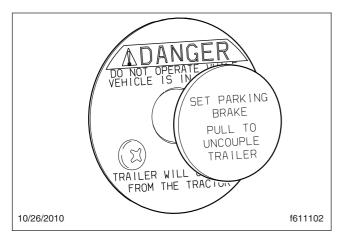
Fig. 18.10, Air-Actuated Kingpin Release Valve
