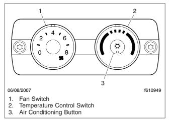
Fig. 8.5, Sleeper Climate Control Panel
