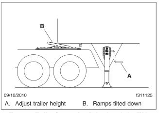
Fig. 18.5, Trailer Connection Point, Low-Lube Fifth Wheel
