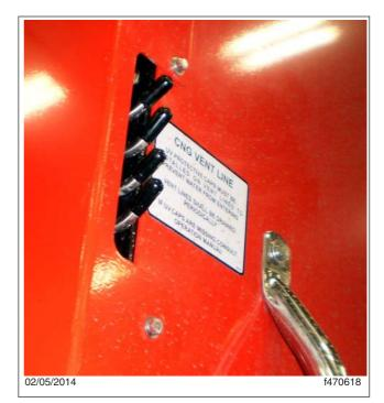
Fig. 21.8, CNG Vent Line Caps
