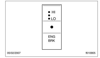
Fig. 13.6, Engine Brake Level Switch
