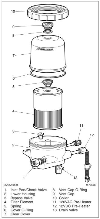
Fig. 21.16, DAVCO Fuel/Water Separator (Fuel Pro 482 shown)
