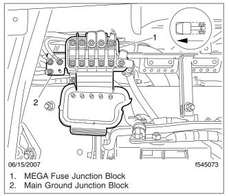
Fig. 3.2, EPA07 MEGA Fuse Junction Block
