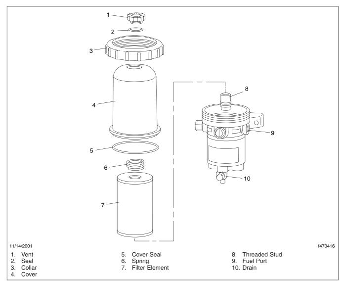
Fig. 24.2, Davco Model 232 and 233 Fuel/Water Separator
