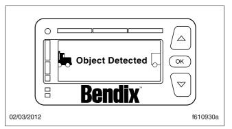
Fig. 6.9, Object Detected Alert
