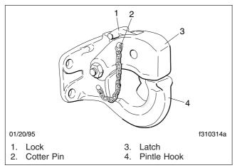
Fig. 19.1, Holland PH-T-60-AL Trailer Coupling
