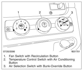
Fig. 5.36, Cab Climate Control Panel
