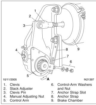
Fig. 21.2, Haldex Automatic Slack Adjuster
