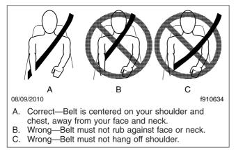
Fig. 7.10, Proper Shoulder Strap Fit
