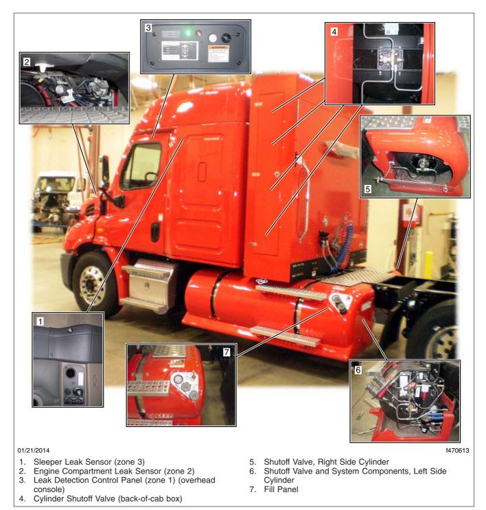
Fig. 25.1, CNG Component Locations
