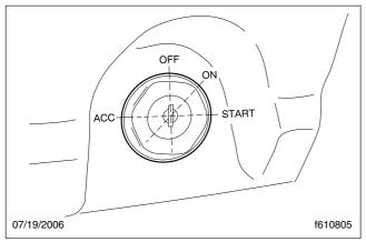
Fig. 25.7, Ignition Switch Positions
