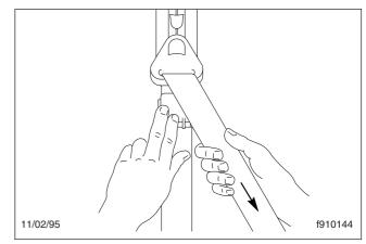
Fig. 7.12, Locking the Komfort Latch
