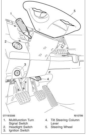
Fig. 5.40, Steering Column and Left Panel Controls
