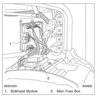
Fig. 2.11, Location of the Main Fuse Box
