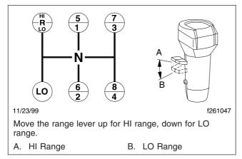
Fig. 8.6, Shift Pattern, 9-Speed Models
