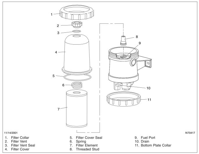
Fig. 13.3, Davco Model 382 Fuel/Water Separator
