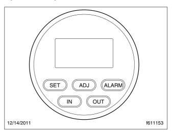
Fig. 3.8, Ambient Temperature Gauge
