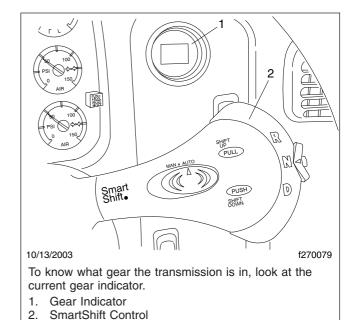
Fig. 8.12, Shift Controls and Indicators, UltraShift Transmissions
