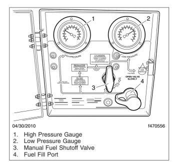
Fig. 11.9, CNG Fuel Panel
