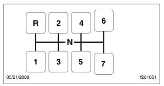
Fig. 8.5, Shift Pattern, 7-Speed T Models
