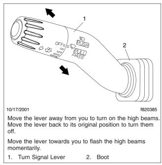
Fig. 4.13, Headlight High Beams
