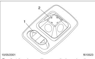
To adjust the mirror position, press the keypad on the door in the direction you want the mirror to move.
