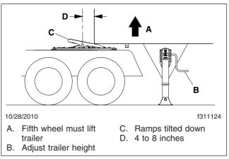
Fig. 10.4, Trailer Connection Point, Standard Fifth Wheel
