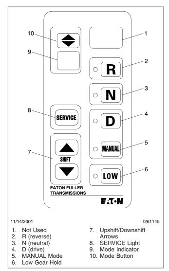
Fig. 8.9, Eaton Push-Button Shift Selector
