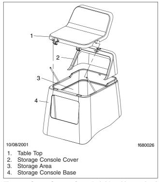
Fig. 5.23, Center Storage Console (with writing surface)
