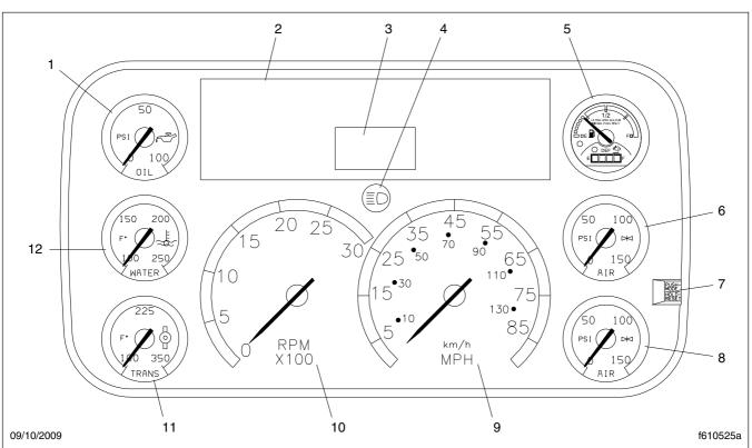
NOTE: This instrument cluster is shown with the U.S. speedometer, which shows miles per hour (mph) more prominently than kilometers per hour (km/h).
