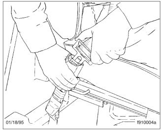
Fig. 5.19, Fastening the Three-Point Belt
