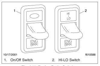
Fig. 4.18, Engine Brake Switches
