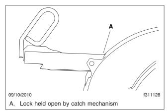
Fig. 10.7, Jost Release Handle Unlocked
