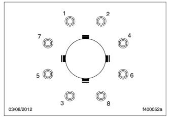
Fig. 11.5, Tightening Pattern, 8-Hole Wheels
