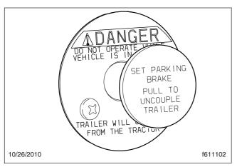
Fig. 10.10, Air-Actuated Kingpin Release Valve
