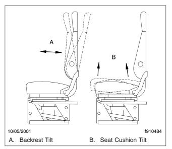
Fig. 5.8, Cushion Tilt Adjustments
