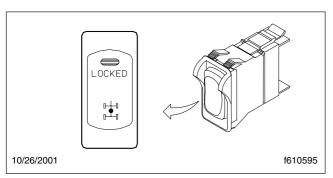
Fig. 4.25, Interaxle Lock Switch
