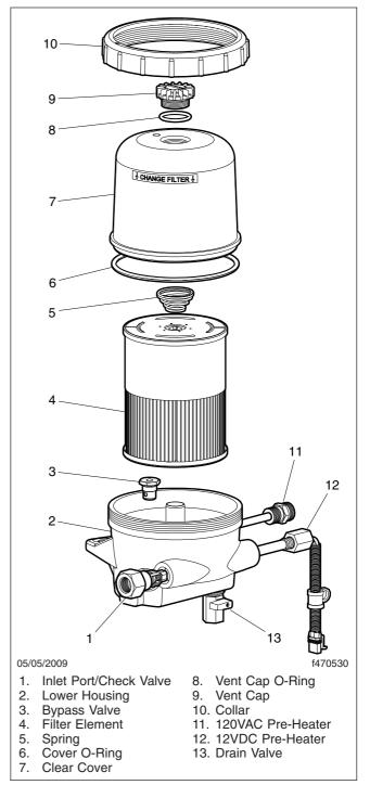
Fig. 11.12, DAVCO Fuel/Water Separator (Fuel Pro 482 shown)
