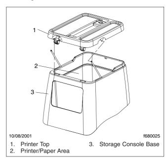
Fig. 5.24, Center Storage Console (printer option)
