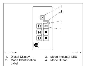
Fig. 8.1, WTEC III Push-Button Shift Selector
