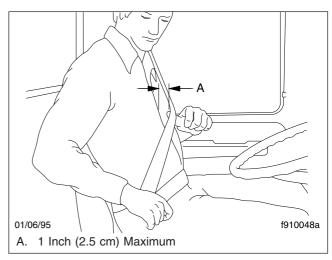
Fig. 5.20, Adjusting Shoulder Harness Clearance, Komfort Latch
