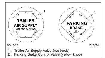
Fig. 4.29, Brake Valve Control Knobs
