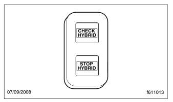
Fig. 15.1, Hybrid System Fault Lamps
