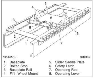
Fig. 10.13, Sliding Fifth Wheel Manual Release, (Holland Simplex)
