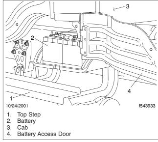
Fig. 2.8, Battery Compartment, Open
