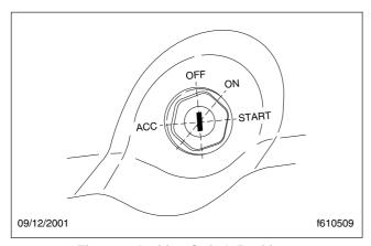
Fig. 16.7, Ignition Switch Positions
