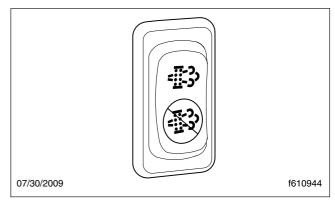
Fig. 7.2, Regen Request/Inhibit Switch
