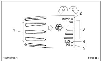
Rotate the control dial away from you to turn the wipers on, or speed them up.
