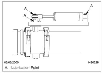
Fig. 7.20, Pacbrake Exhaust Brake and Air Cylinder
