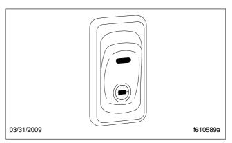
Fig. 7.19, Exhaust Brake Switch
