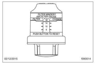
Fig. 3.6, Air Intake Restriction Indicator
