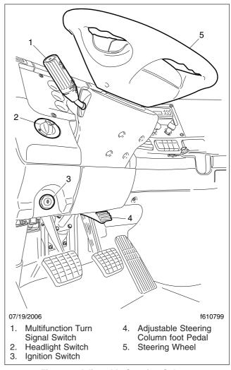
Fig. 4.32, Adjustable Steering Column
