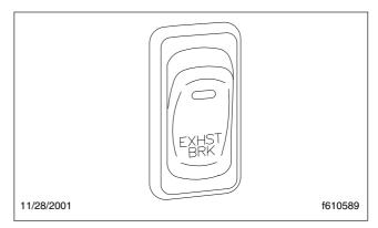
Fig. 7.18, Exhaust Brake Switch
