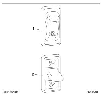
To turn cruise control on, press the upper half of the On/ Off switch. To turn cruise control off, press the lower half of the On/Off switch.
