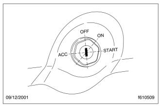
Fig. 4.1, Ignition Switch Positions
