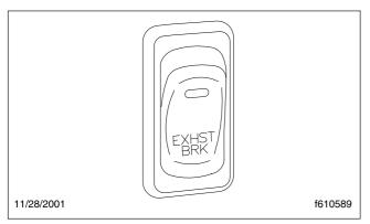
Fig. 4.19, Exhaust Brake Switch
