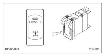
Fig. 8.23, Interaxle Lock Switch
