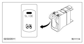
Fig. 10.14, Air-Slide Switch
