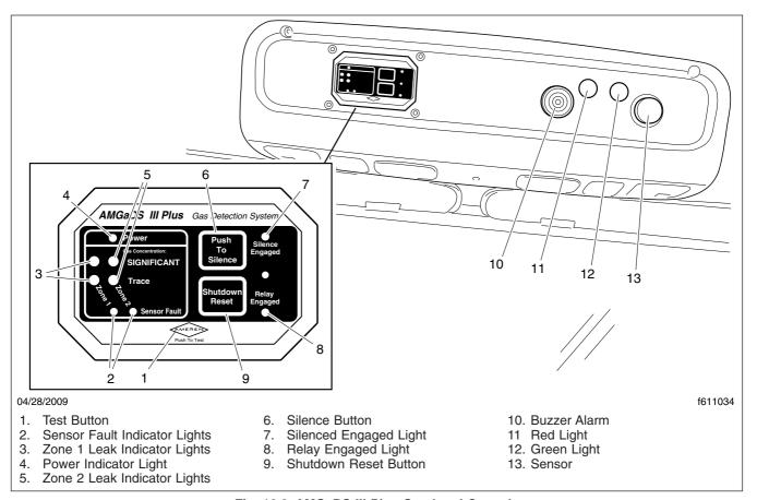
Fig. 16.6, AMGaDS III Plus Overhead Console
