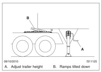
Fig. 10.5, Trailer Connection Point, Low-Lube Fifth Wheel
