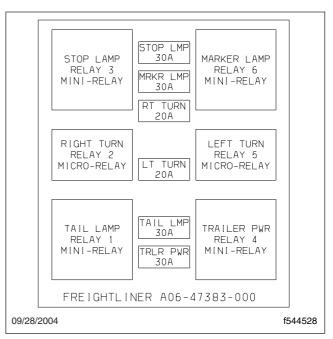
Fig. 2.13, Trailer Fuse Box Diagram
