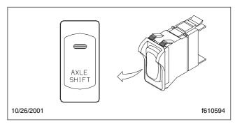
Fig. 4.26, Axle Shift Switch
