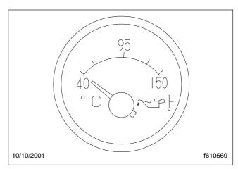
Fig. 3.11, Engine Oil Temperature Gauge
