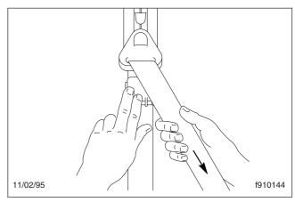
Fig. 5.21, Locking the Komfort Latch
