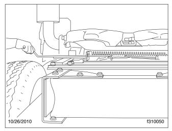
Fig. 10.12, Releasing the Sliding Fifth Wheel, (Fontaine)
