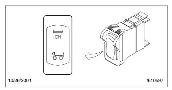
Fig. 4.33, Suspension Dump Switch
