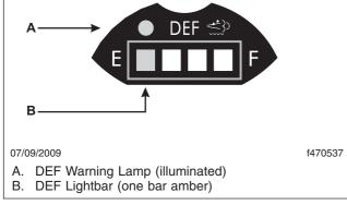
Fig. 7.11, DEF Level Low Initial Warning
