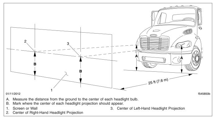
Fig. 14.2, Headlight Aiming Screen/Wall
