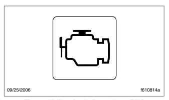
Fig. 7.5, Malfunction Indicator Lamp (MIL)
