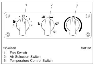
Fig. 4.35, HVAC Climate Control Panel, Standard
