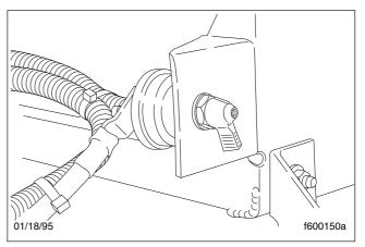
Fig. 2.9, Cab (Battery) Isolation Switch
