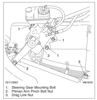
Fig. 11.13, Steering Gear Fasteners
