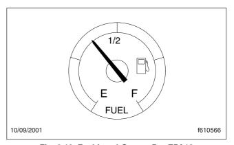
Fig. 3.12, Fuel Level Gauge, Pre-EPA10
