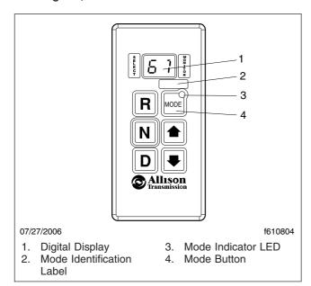
Fig. 8.2, Fourth Generation Push-Button Shift Selector
