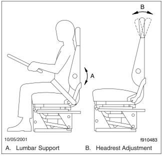
Fig. 5.7, Lumbar Support and Headrest Adjustment
