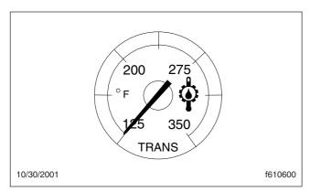
Fig. 3.15, Transmission Fluid Temperature Gauge
