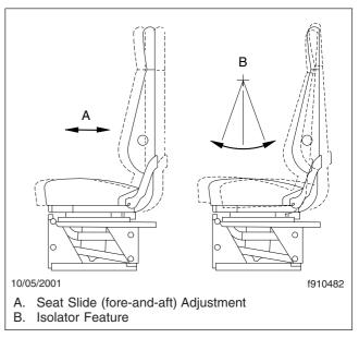
Fig. 5.6, Seat Slide Adjustment and Isolator Feature
