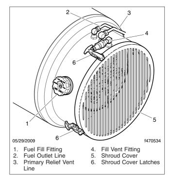
Fig. 16.2, LNG Fuel Tank
