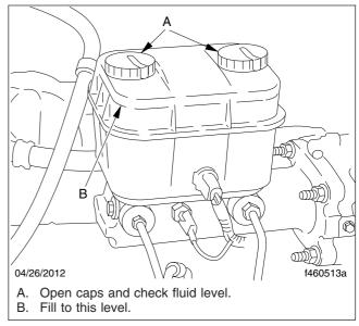
Fig. 9.4, Hydraulic Brake Reservoir
