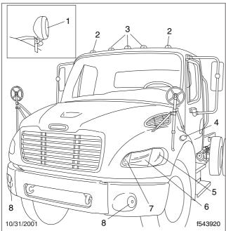
NOTE: The parking lights, front clearance lights, and taillights all function as turn signals.
