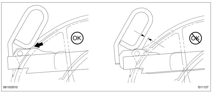
Fig. 10.8, Jost Release Handle Locked
