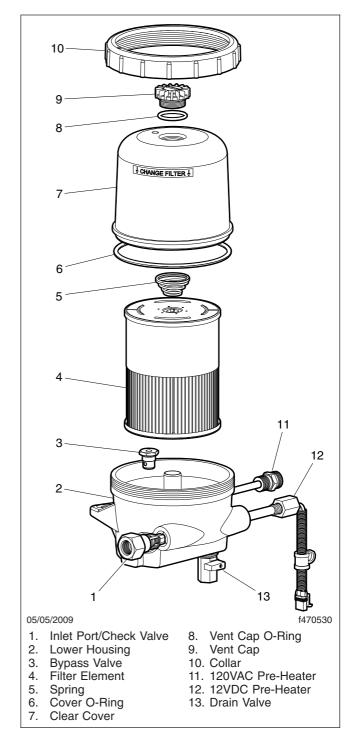
Fig. 21.13, DAVCO Fuel/Water Separator (Fuel Pro 482 shown)
