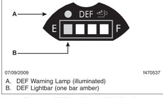
Fig. 11.11, DEF Level Low Initial Warning
