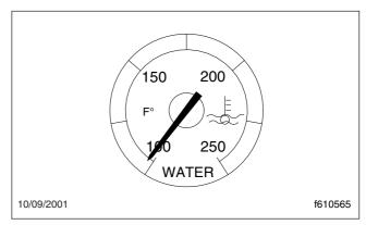
Fig. 4.7, Coolant Temperature Gauge
