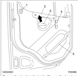
To open the door from the inside, lift up on the door lever (arrow).
