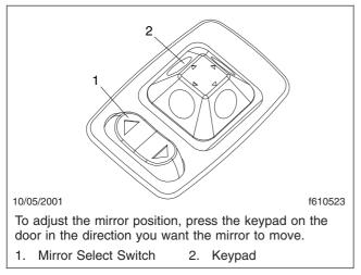
Fig. 8.4, Power Mirror Switch Pad
