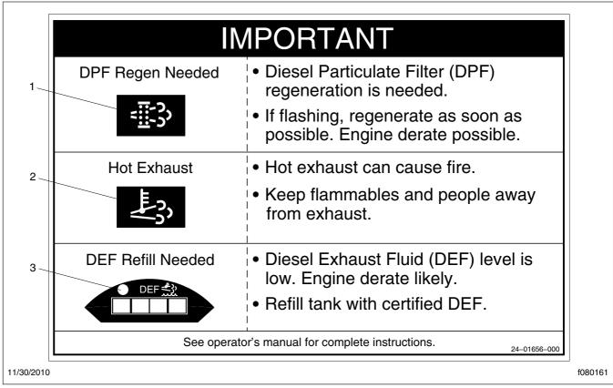
Fig. 11.3, Warning Lamp Decal, Sun Visor
