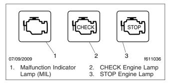
Fig. 10.1, Engine Warning Lights
