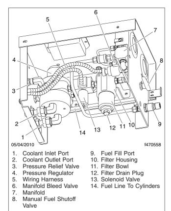
Fig. 21.17, CNG Fuel Panel Components
