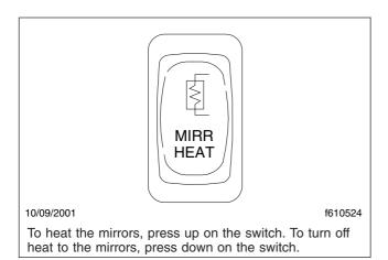
Fig. 8.3, Mirror Heat Switch
