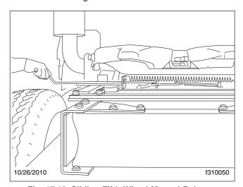
Fig. 17.12, Sliding Fifth Wheel Manual Release, Fontaine
