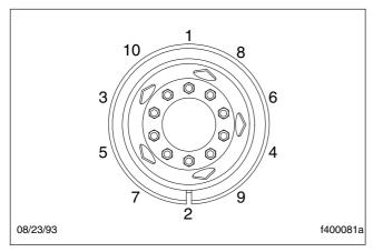
Fig. 21.4, Tightening Pattern, 10-Hole Wheels
