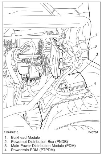
Fig. 21.7, Visible Engine Wiring
