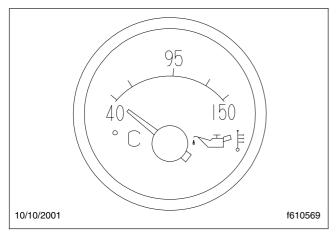
Fig. 4.10, Engine Oil Temperature Gauge
