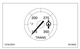
Fig. 4.13, Transmission Fluid Temperature Gauge
