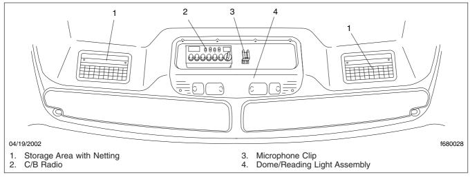
Fig. 4.14, Overhead Instrument Panel
