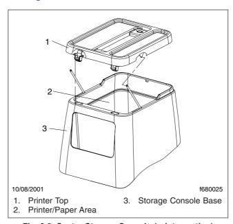
Fig. 8.2, Center Storage Console (printer option)
