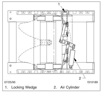
Fig. 17.15, Air-Operated Sliding Fifth Wheel, Fontaine
