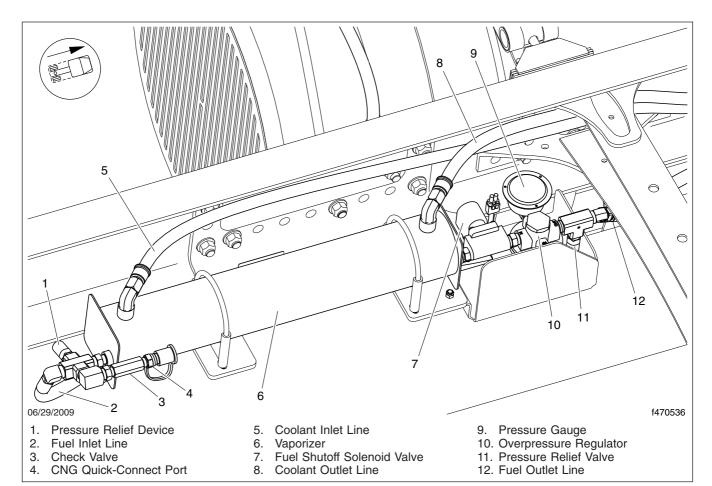
Fig. 21.11, LNG Vaporizer Assembly
