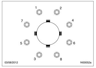
Fig. 21.5, Tightening Pattern, 8-Hole Wheels
