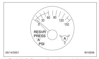
Fig. 4.12, Air Pressure Gauge (reservoir A shown)
