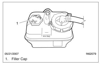
Fig. 21.6, Power Steering Fluid Reservoir
