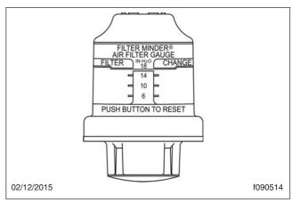
Fig. 4.5, Air Intake Restriction Indicator
