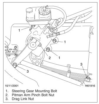
Fig. 21.14, Steering Gear Fasteners
