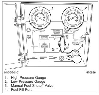
Fig. 21.10, CNG Fuel Panel
