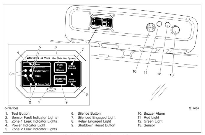
Fig. 19.6, AMGaDS III Plus Overhead Console
