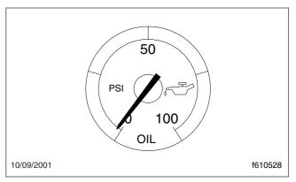
Fig. 4.9, Engine Oil Pressure Gauge
