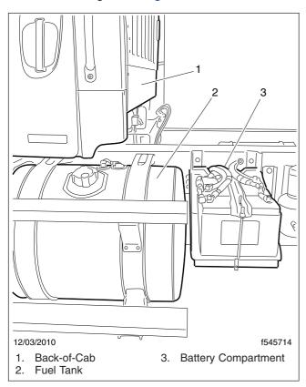
Fig. 21.15, Standard Battery Compartment Location
