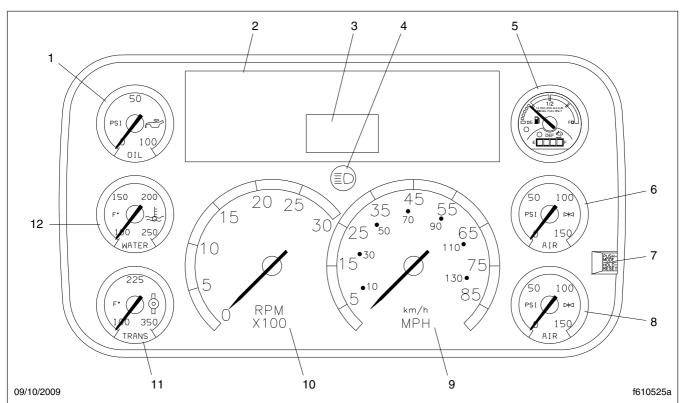
NOTE: This instrument cluster is shown with the U.S. speedometer, which shows miles per hour (mph) more prominently than kilometers per hour (km/h).
