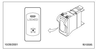
Fig. 5.20, Interaxle Lock Switch
