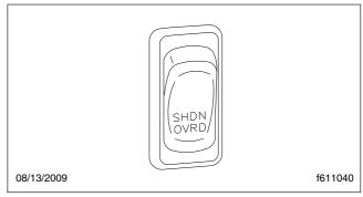
Fig. 10.2, Shutdown Override Switch
