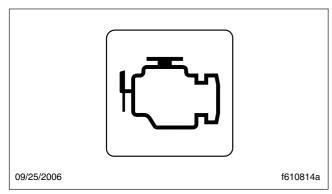
Fig. 11.5, Malfunction Indicator Lamp (MIL)
